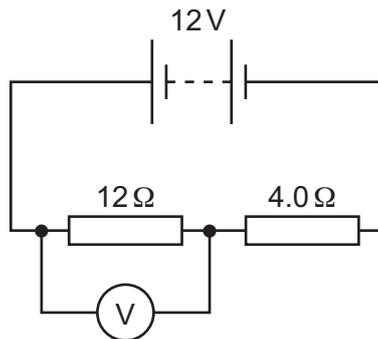
There is a voltmeter connected across the  $12\ \Omega$  resistor.
